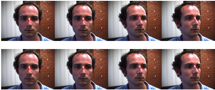
Fig. 7. Comparison of intensity-based tracker to hybrid tracker. The top row is the intensity tracker and the bottom is the hybrid tracker for the same sequence. The intensity-based tracker is more sensitive to the strong reflection.
